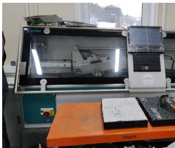
Fig. 2. Production of asphalt concrete samples Fig. 3. Testing of asphalt concrete samples according to GOST R 58406.2-2020
