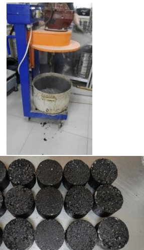
Fig. 2. Production of asphalt concrete samples
