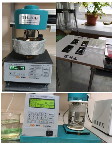
Fig. 1. Testing of bitumen grade BND 700/100
