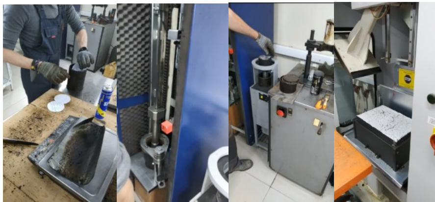
Fig. 3. Preparation of asphalt concrete samples by GOST R 58406.2-2020
