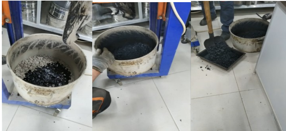
Fig. 2. Production of asphalt concrete mixture of the specified composition
