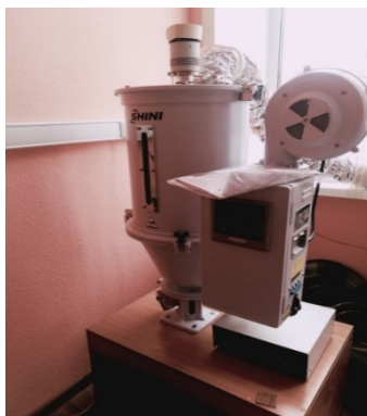
Fig. 1. The exterior of a drying unit with ultrasonic dryer
