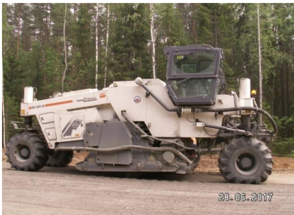
Fig. 1. Wirtgen 2500 recycler during an overhaul of road surface in Yaroslavl region
