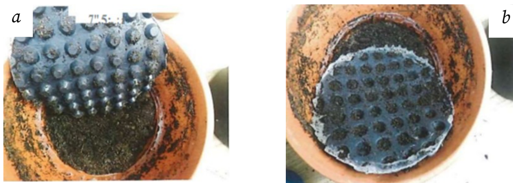
Fig. 9. Testing of profiled membranes for resistance to root – proof: a , b – the sample of the profiled membrane did not allow the roots to germinate
