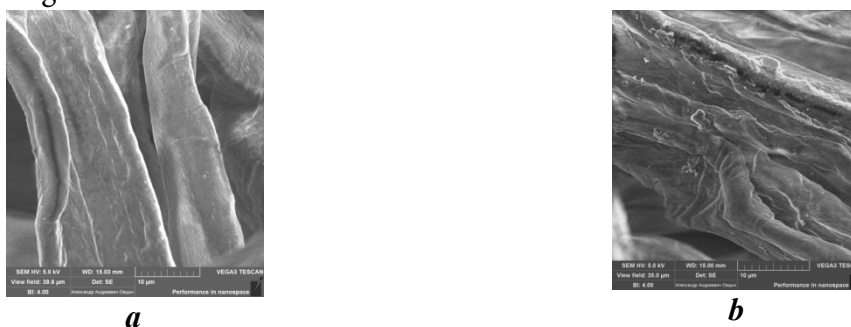
Fig. 6. SEM images of the surface of sorbents: a - original cellulose; b - cellulose modified with glycine
